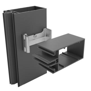
Die-cast aluminum bracket for sequential assembly of curtain wall systems. This system eliminates the time-consuming installation by screws and allows a quick and accurate fastening thanks to the holes drilled on the mullion. With fixed anchoring buttons and safety screw. **Patented.**
