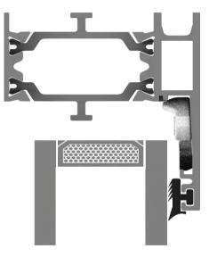
Die-cast aluminum corner joint with alignment and tightening function. Thanks to the two conical slides tightened with a simple slotted screwdriver, it aligns and closes the profile flawlessly. It can be installed on assembled profiles and, if necessary, easily disassembled. No profile processing is required. It has specific glue channels to guarantee perfect sealing and greater strength while avoiding any waste or spill. **Patented**.
