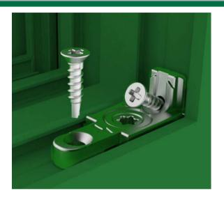
Fastening and aligning T-Joint for instant fixing of Euro groove profiles. Die cast zama with adjustable cam and tightening screws. Specifically designed for muntin and mullion assembly. Fixing achieved after the profile is assembled. No profile processing. No glazing bead interference.
